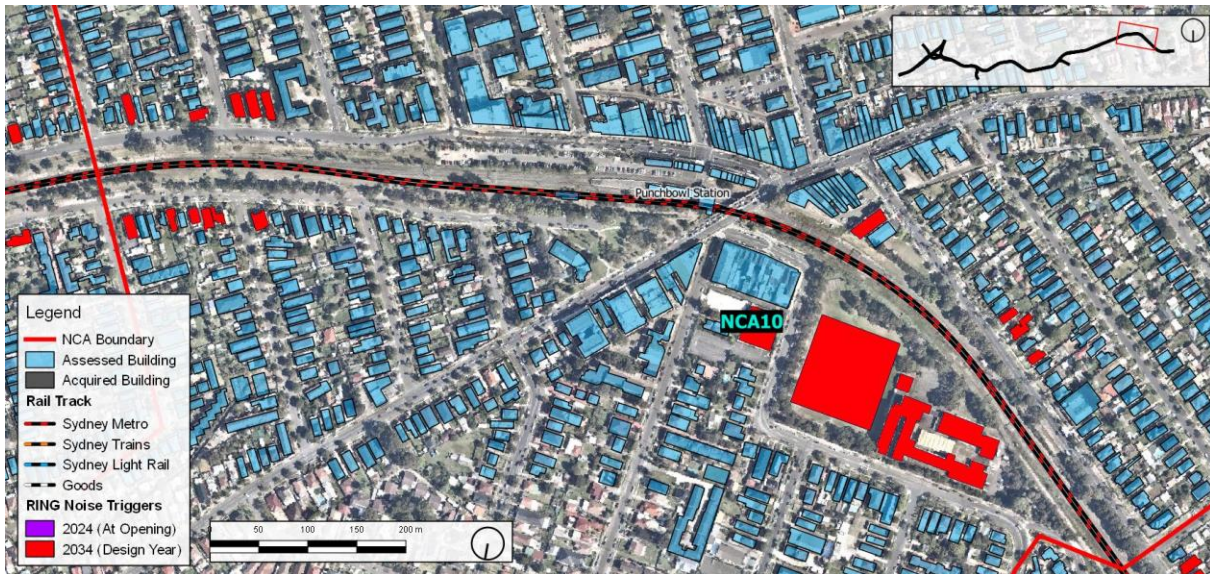
Figure 66 NCA10 Locations Triggerred for Consideration of Noise Mitigation
