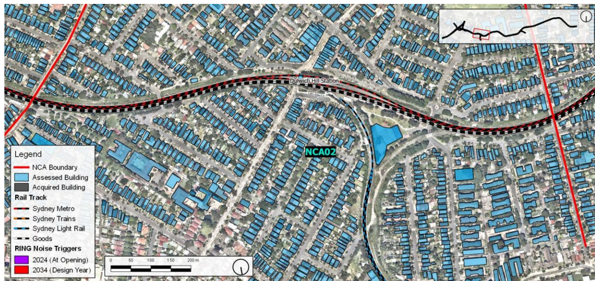
Figure 57 NCA02 Locations Triggered for Consideration of Noise Mitigation
