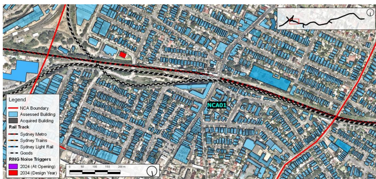
Figure 56 NCA01 Locations Triggered for Consideration of Noise Mitigation
