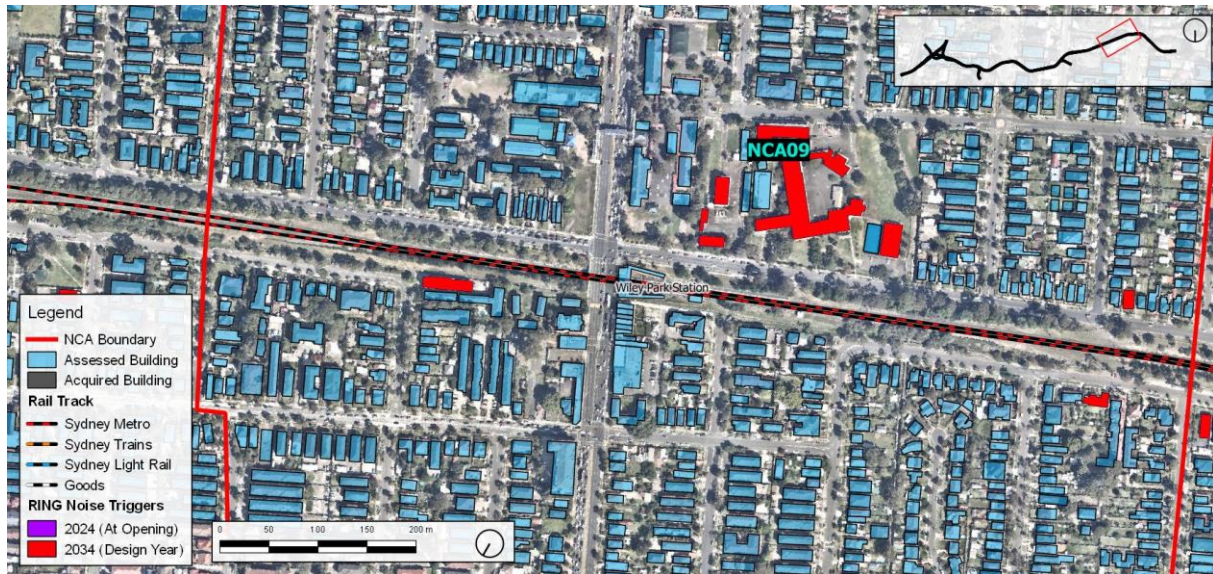
Figure 65 NCA09 Locations Triggerred for Consideration of Noise Mitigation
