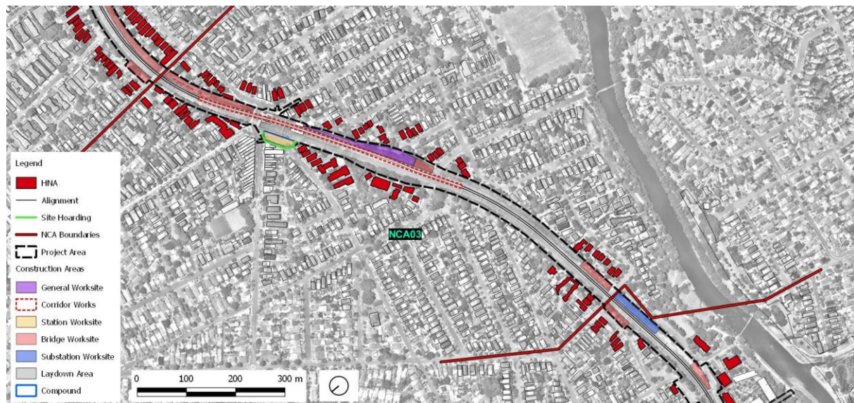
Figure 20 Highly Noise Affected Residential Receivers
