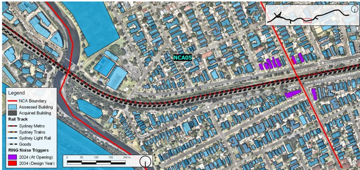
Figure 61 NCA05 Locations Triggered for Consideration of Noise Mitigation
