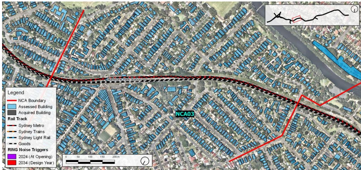
Figure 58 NCA03 Locations Triggered for Consideration of Noise Mitigation
