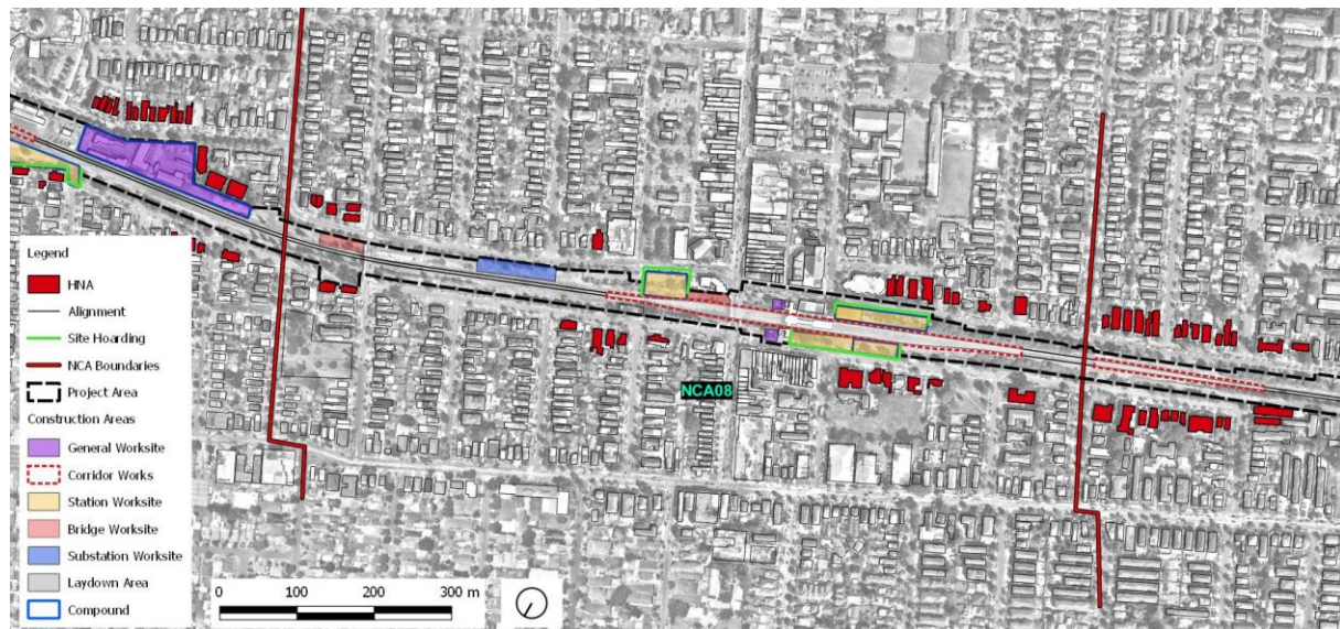
Figure 39 Highly Noise Affected Residential Receivers
