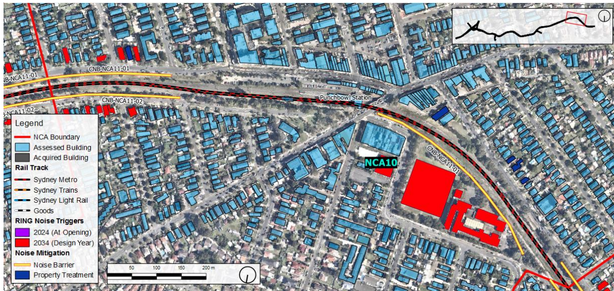
Figure 77 Recommended Airborne Noise Mitigation - Punchbowl Precinct
