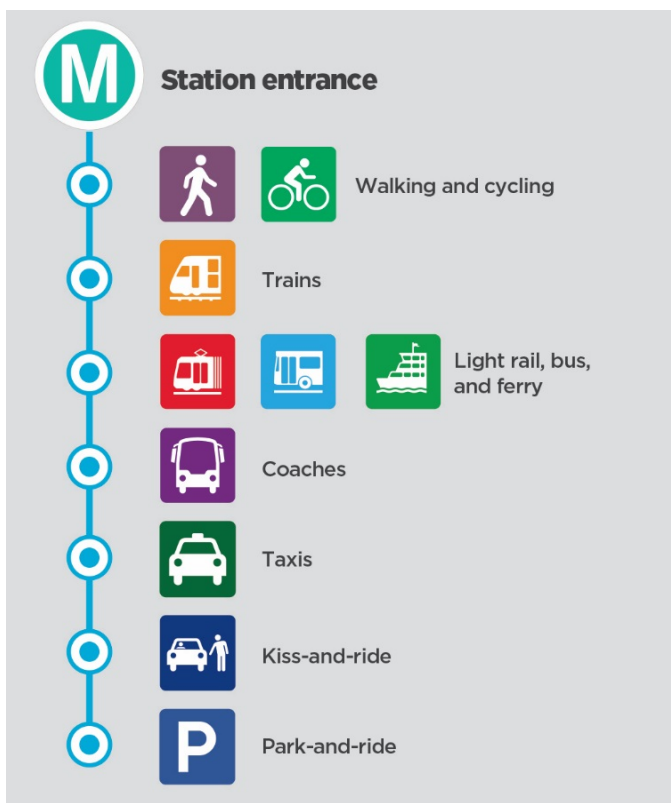
Figure 7.1 Station access hierarchy
