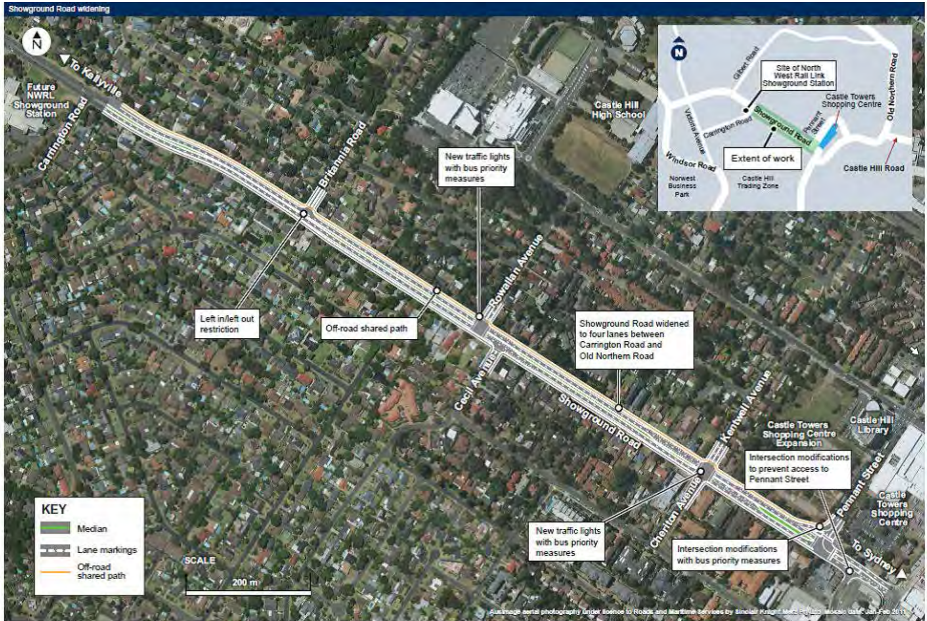
Figure 5.2 Showground Road upgrade by RMS. Source: RMS
