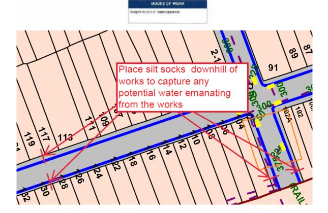
Note: For the duration of the works silt control socks are to be used at storm water inlets downhill from the works
