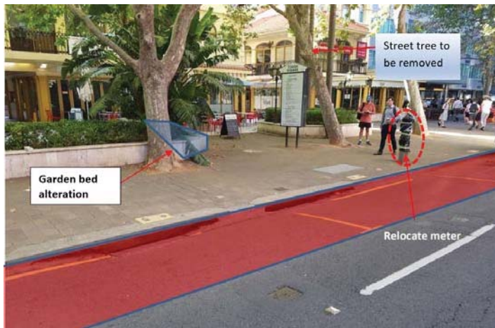
FIGURE 3 WORKS TO FACILITATE SITE ACCESS/ EGRESS
