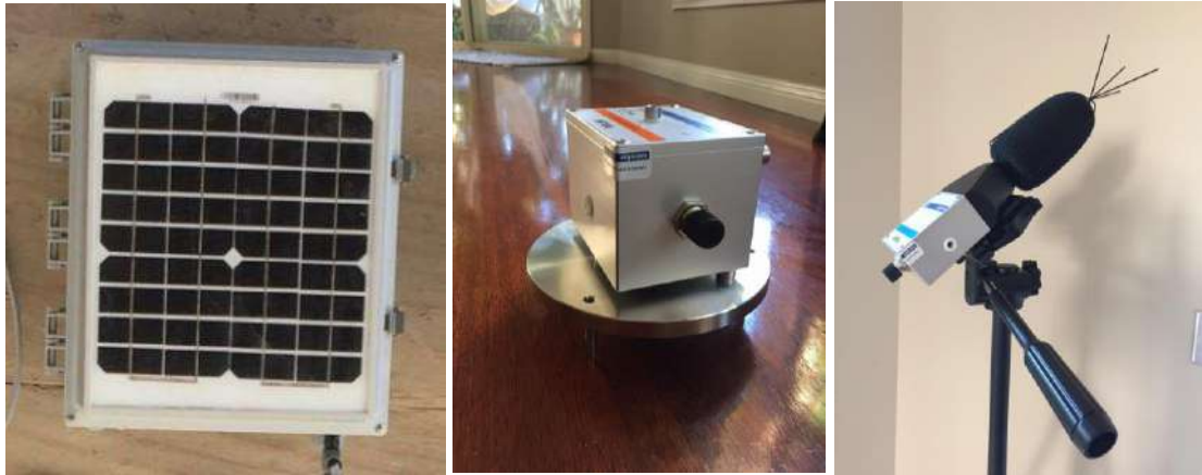
Figure 1 The components of the vibration monitoring; the logger (left), geophone set on comfort plate (centre) and microphone (left).
