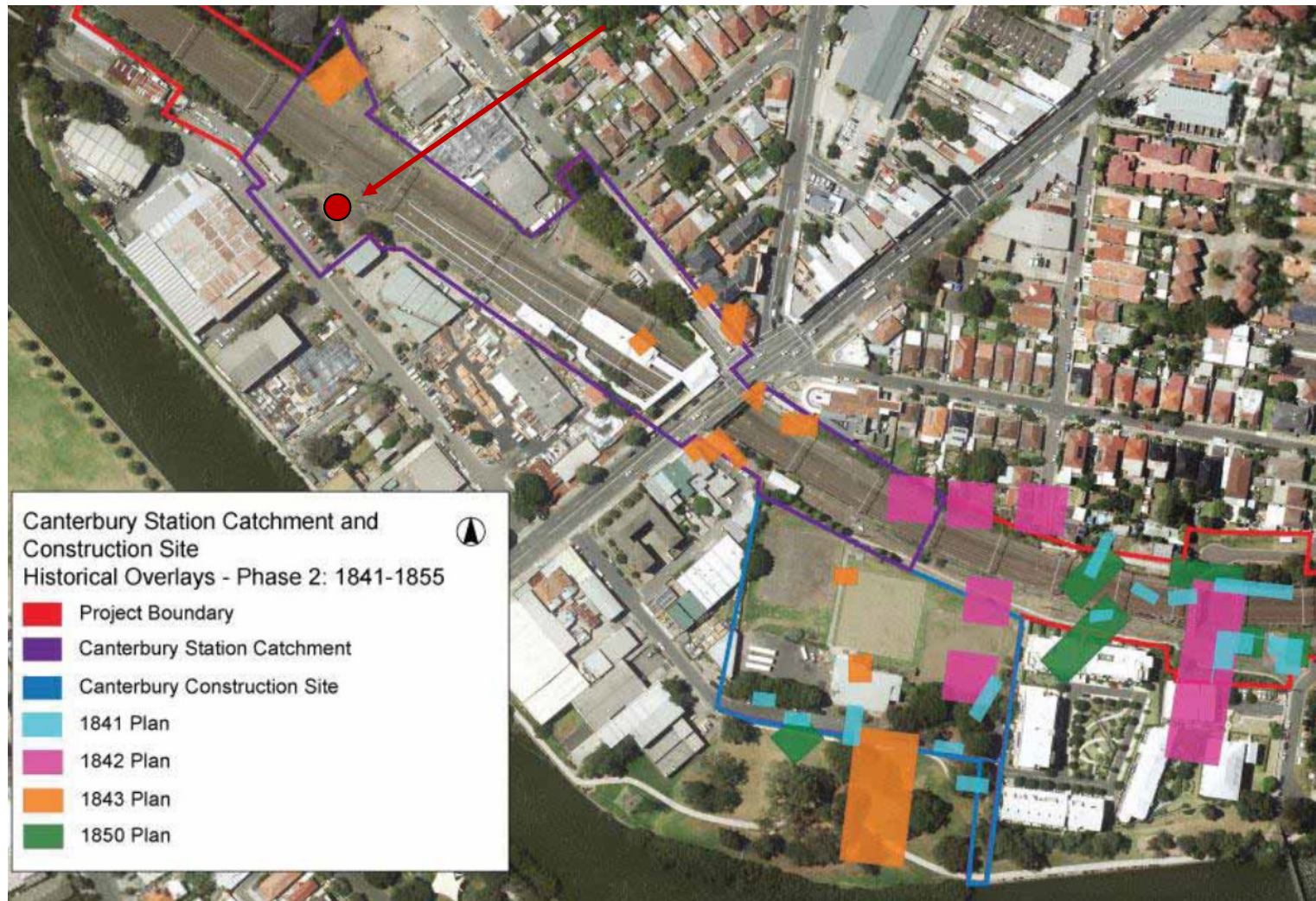
Figure 3: Historical overlay for Canterbury Station Catchment for Phase 2 (1841 – 1855), location of soil resistivity location indicated with red circle / red arrow
