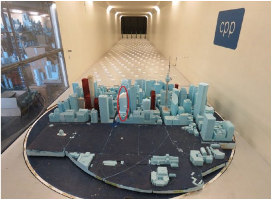
Figure 87 – Wind tunnel testing models used to determine the proposed wind impact (site in red circle)
