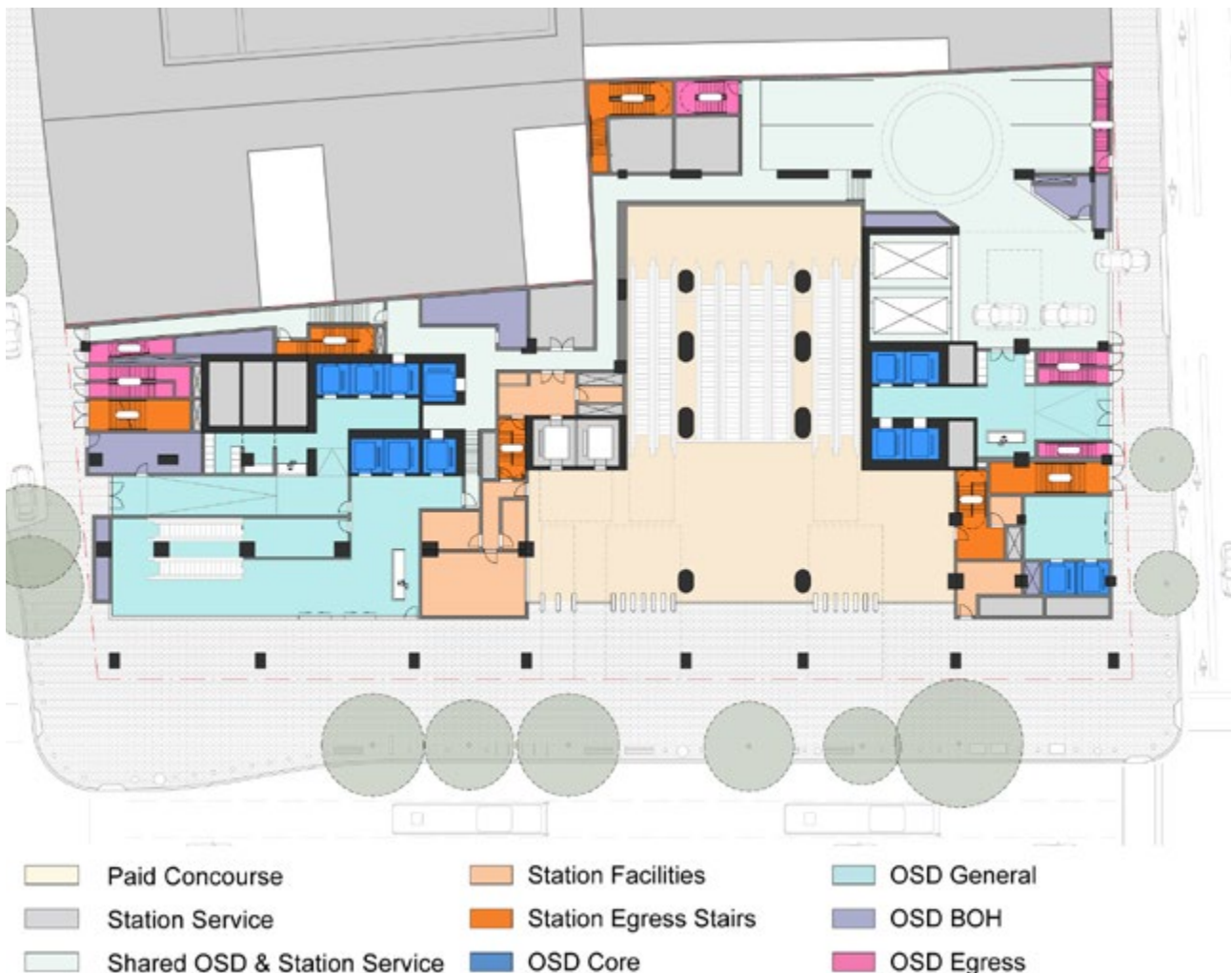
Figure 44 – Indicative ground floor plan, with metro pedestrian access (yellow), OSD pedestrian access (blue) and shared loading access (grey)
