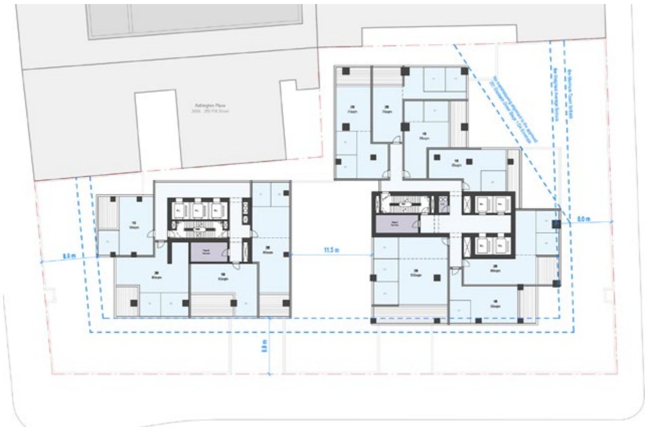
Figure 79 – Floor plan of a scheme comprising two towers, demonstrating a potential interface between each building
