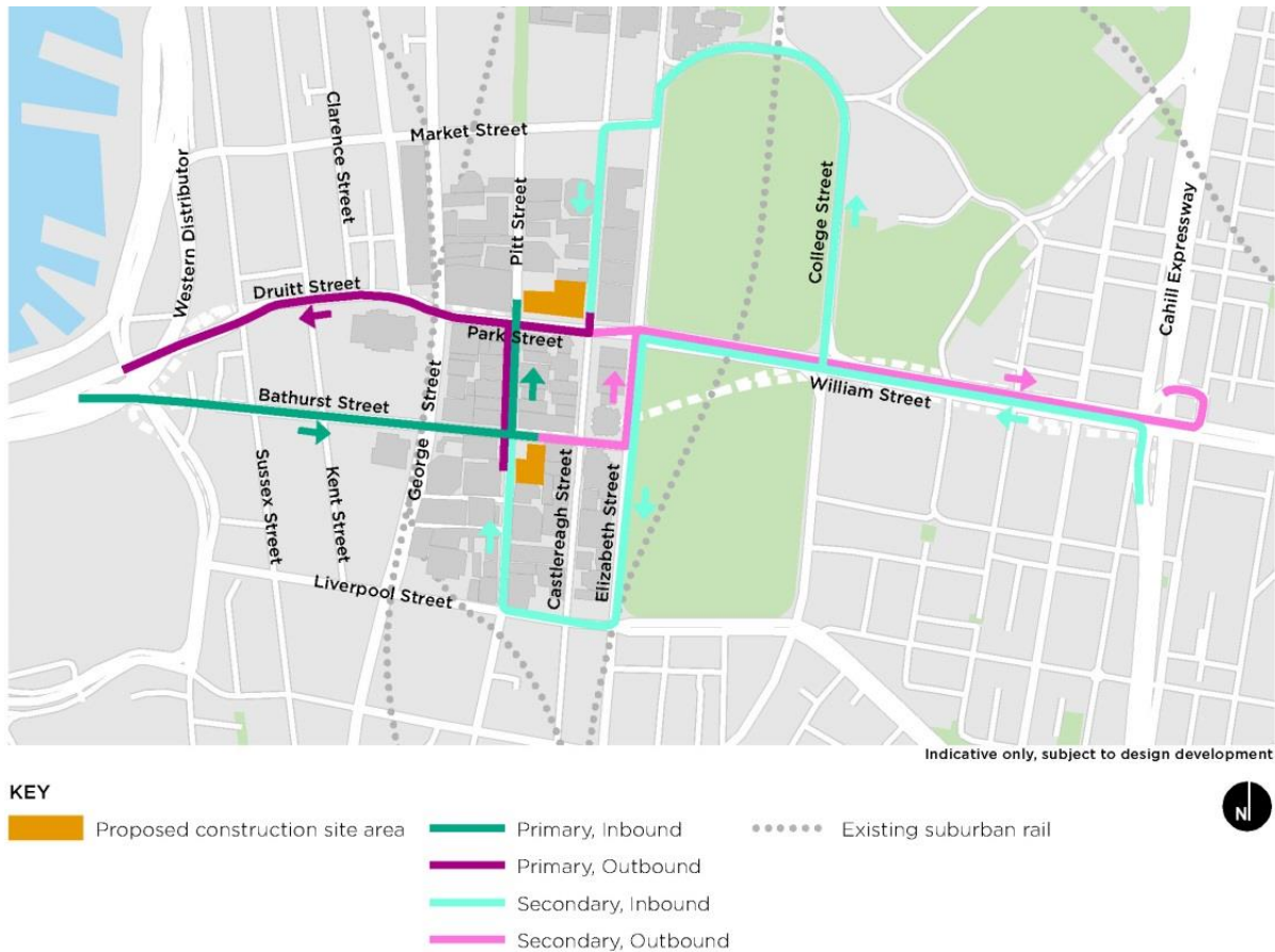
Figure 8: CSSI construction haulage routes, Pitt Street
