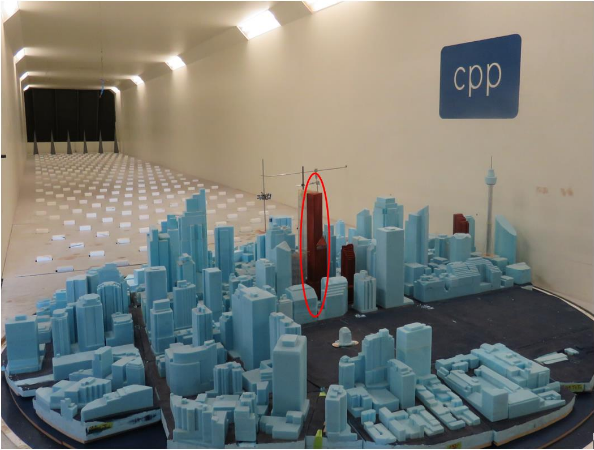
Figure 18: Proposed Sydney Metro – over station development model in the wind tunnel viewed from the east.
