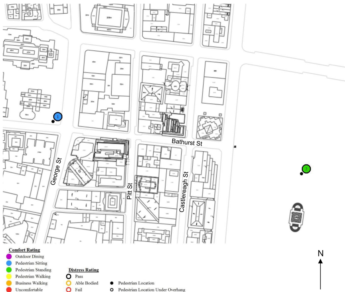
Figure 20: Pedestrian wind speed measurement locations with comfort/distress ratings – Remote locations.
