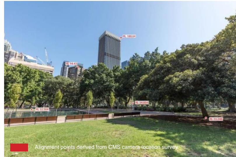
Original photograph with surveyed alignment points
