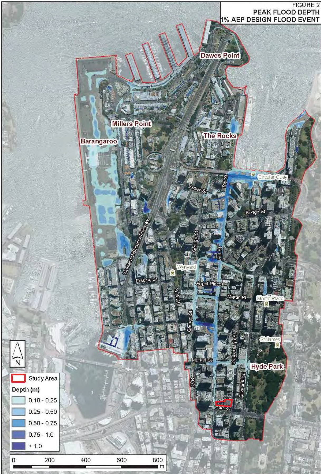
Figure C1 – 100 year ARI Flood Depth
