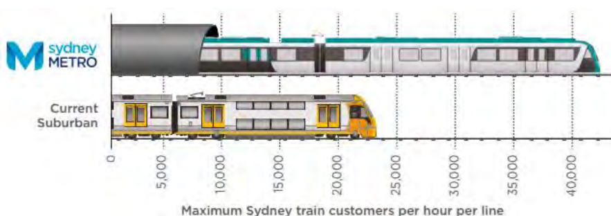
Figure 3 – Capacity of Sydney Metro by comparison to current suburban train lines
