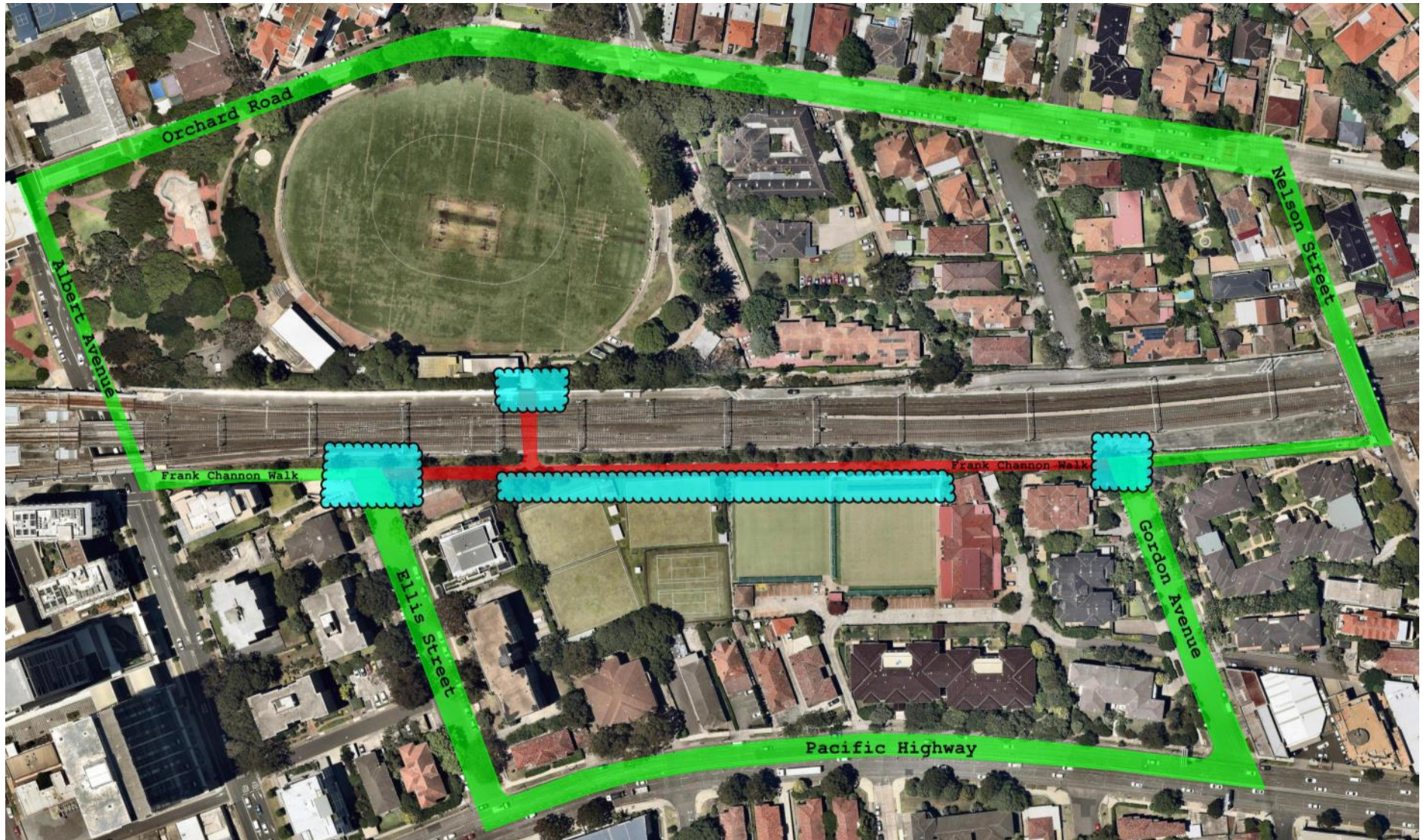
Areas of barricading, fencing and shade cloth surrounding walkway
