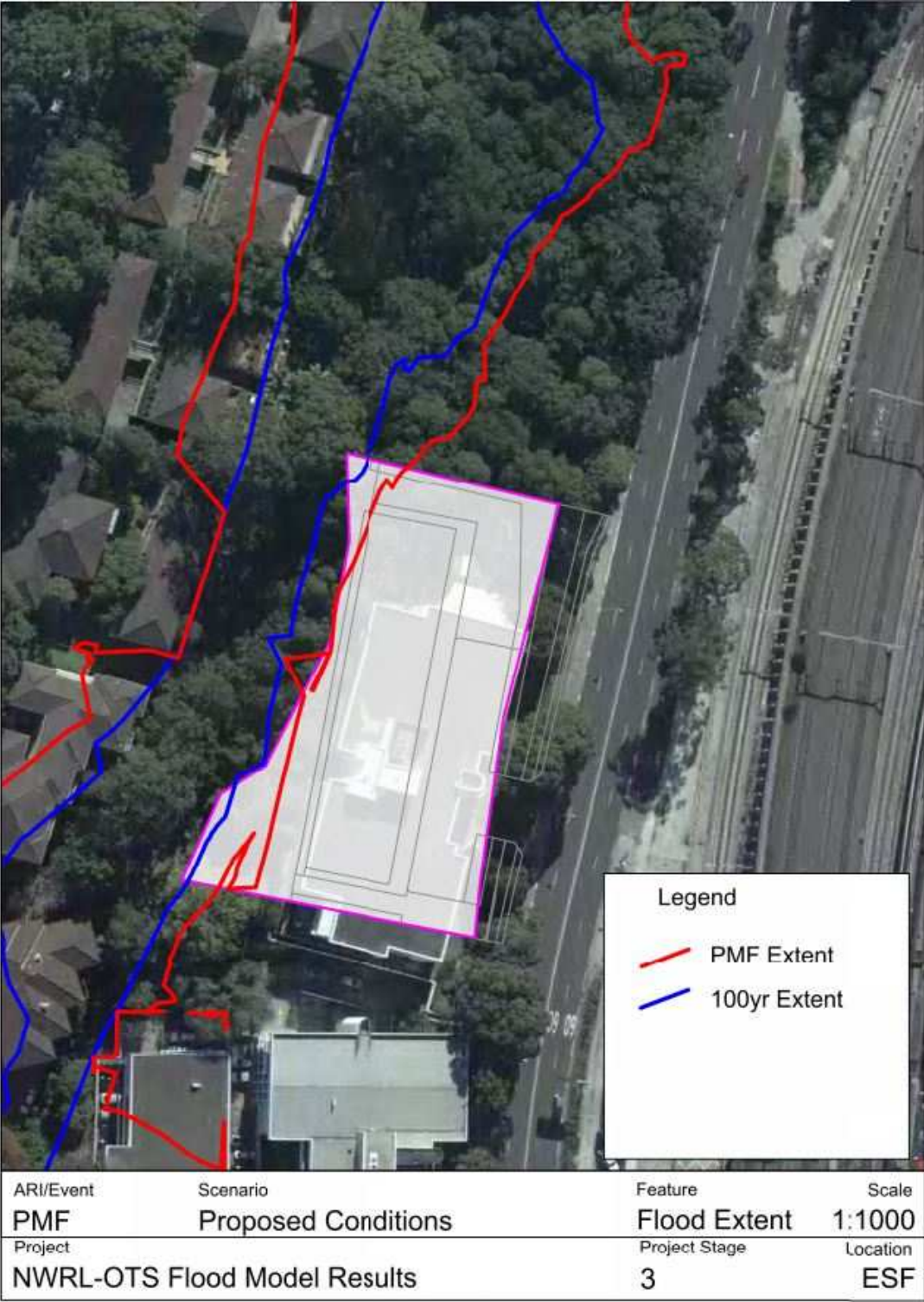
Figure 13 Epping Flood Extents under Proposed Conditions (PMF and 100 year including Climate Change)
