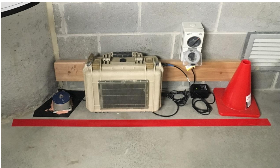
Photo 4.3: Example Vibration Monitoring Setup
