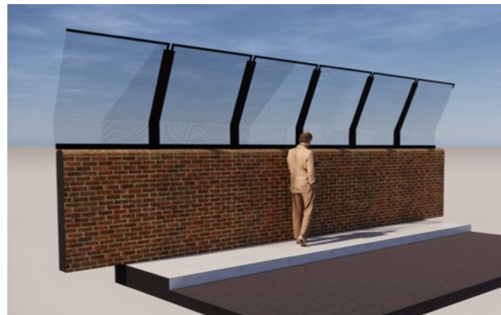
Figure 4.27 Typical Type 1 vertical protection screens
