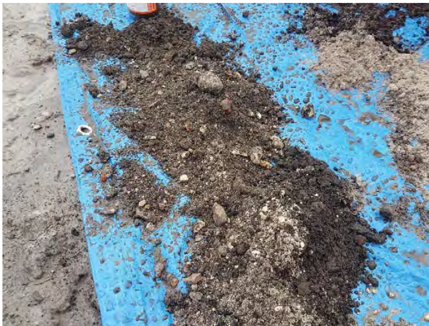
Photograph No.: 3 Description: Fill material at SRT-BH416 at from 0.25 to 0.5 mbgl.
