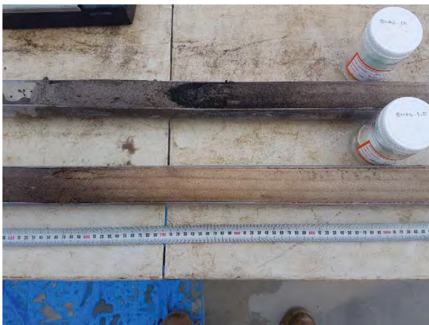
Photograph No.: 4 Description: Push tube splits from 1.5 to 3.2 mbgl at SRT-BH416.
