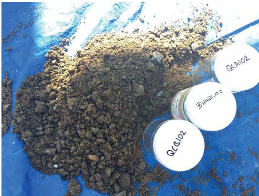
Photograph No.: 5 Description: Fill material at SRT-BH421 at 0.5 mbgl.
