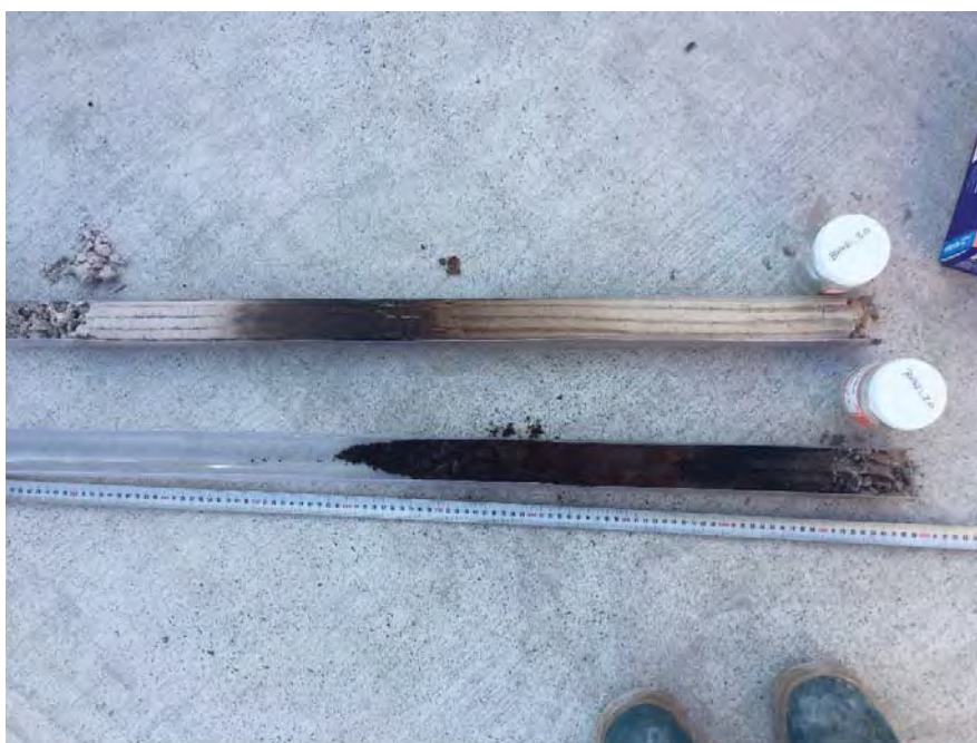
Photograph No.: 6 Description: Push tube splits from 1.5 to 3.2 mbgl SRT-BH421.
