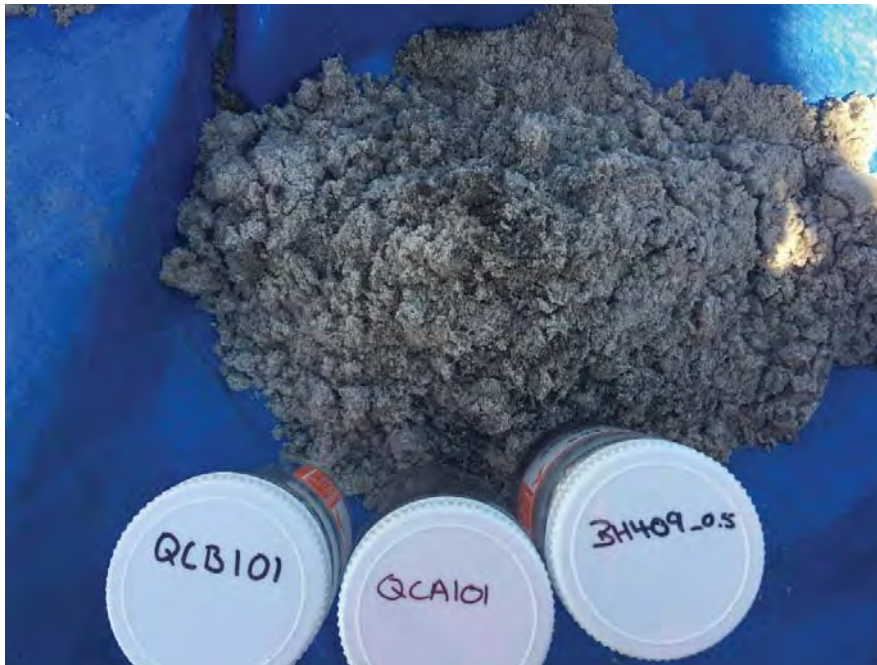
Photograph No.: 1 Description: Re-worked natural material at SRT-BH409 at 0.5 mbgl.
