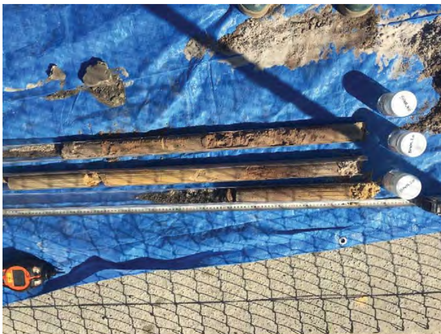
Photograph No.: 2 Description: Push tube splits from 1.5 to 4.2 mbgl SRT-BH409.
