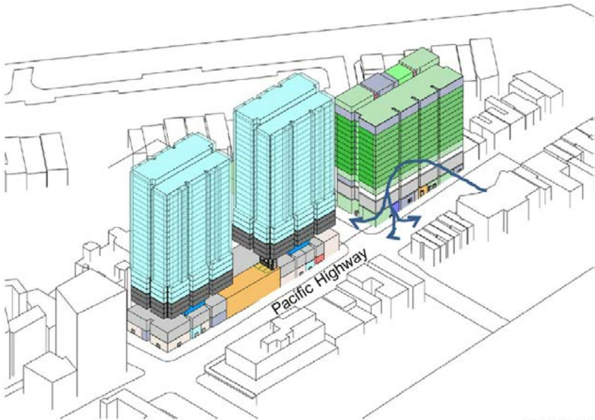
Figure 78 - Downwash caused by winds from the south-west impacting Site B, viewed from the west.
