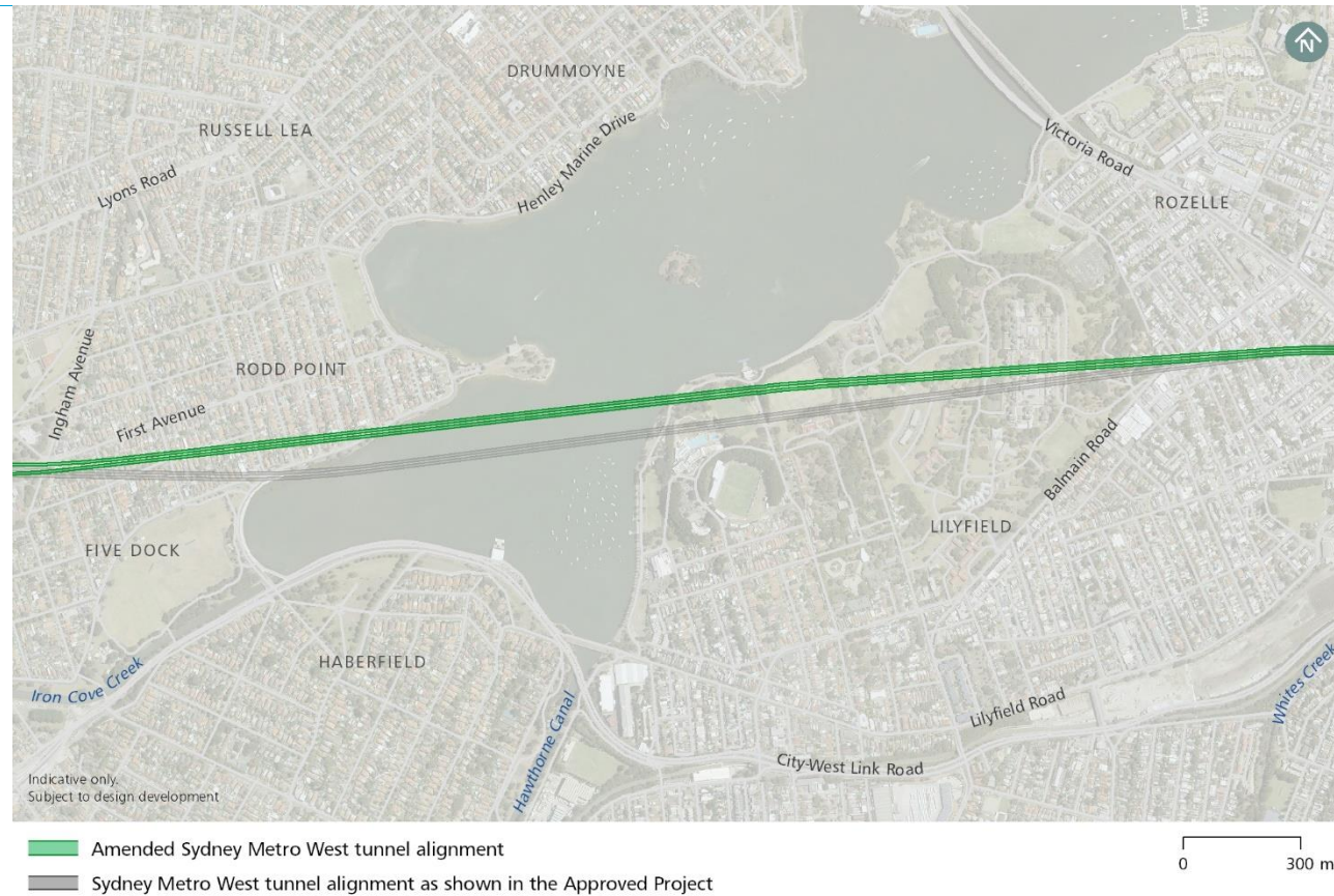
Figure 5: Approved tunnel alignment and proposed tunnel re-alignment between Five Dock Station and The Bays Station
