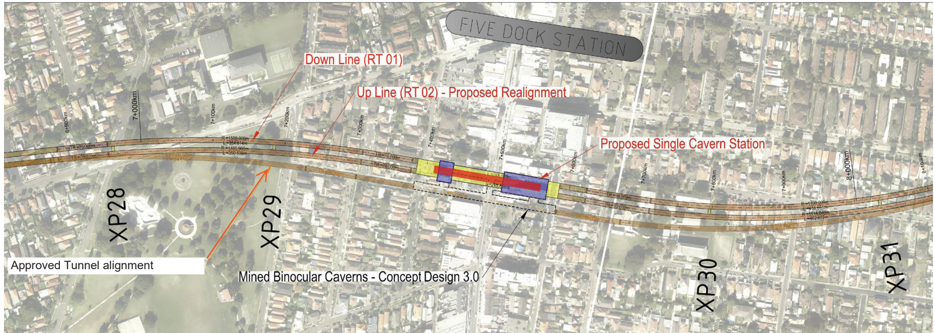
Figure 2 Tunnel alignment change
