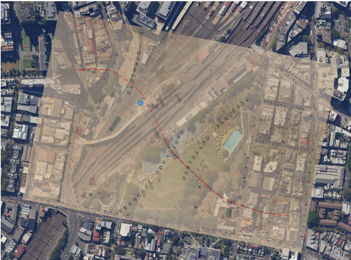
FIGURE 2.18: INDICATIVE LINE OF THE PRINCE ALFRED SEWER LINE (DOTTED RED LINE), WHICH FOLLOWS THE LINE OF A NATURAL WATERCOURSE. MARKED IN BLUE IS THE LOCATION OF THE TURNTABLE ASSOCIATED WITH THE FIRST CENTRAL STATION, WHICH WAS RECENTLY UNCOVERED AS PART OF THE ARCHAEOLOGICAL PROGRAM BEING IMPLEMENTED IN CONJUNCTION WITH CSMW.
