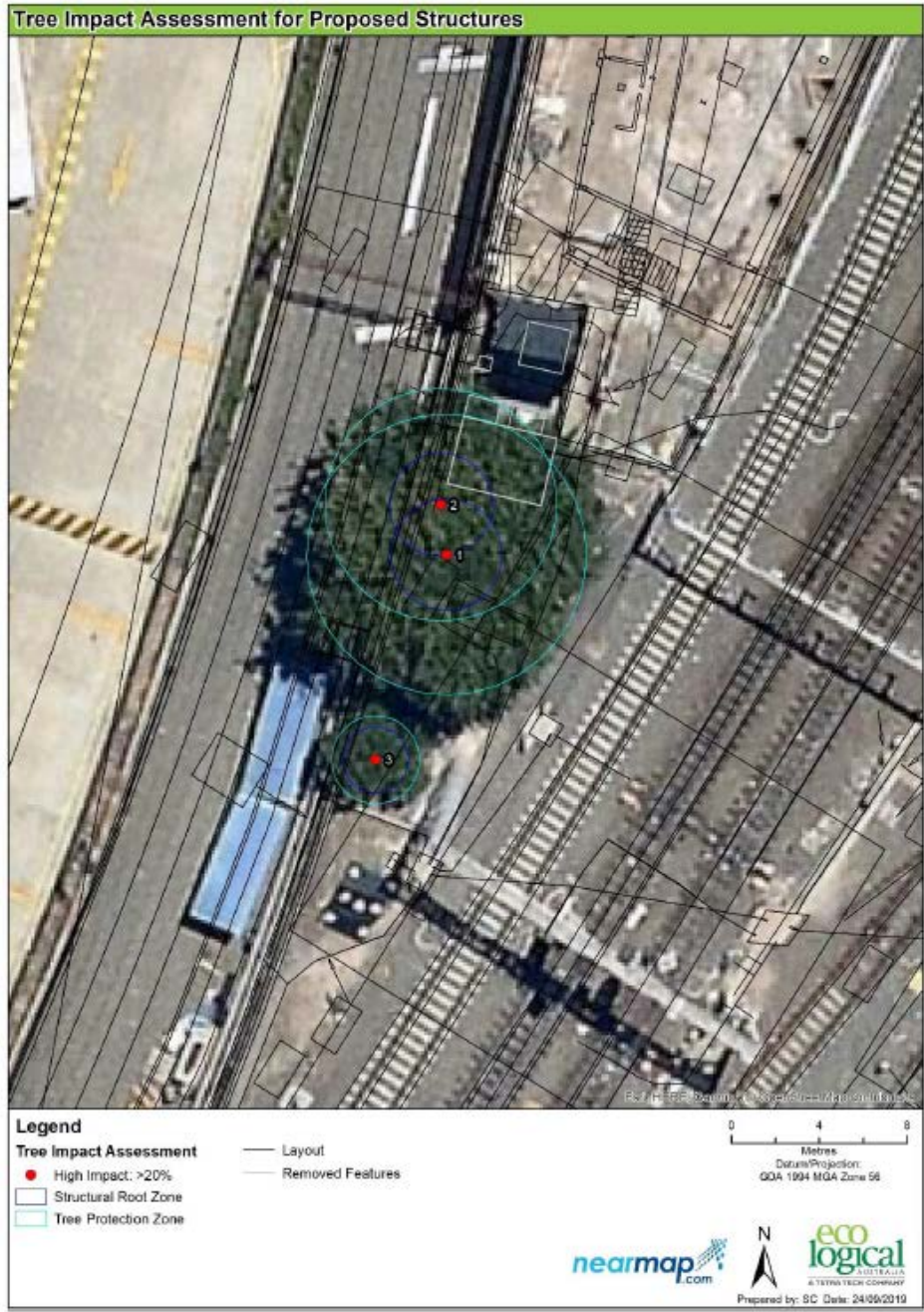
Figure 14.1: Tree impact for CSR and pad mount substation
