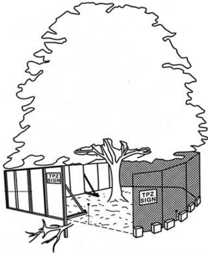
Tree protection fencing
