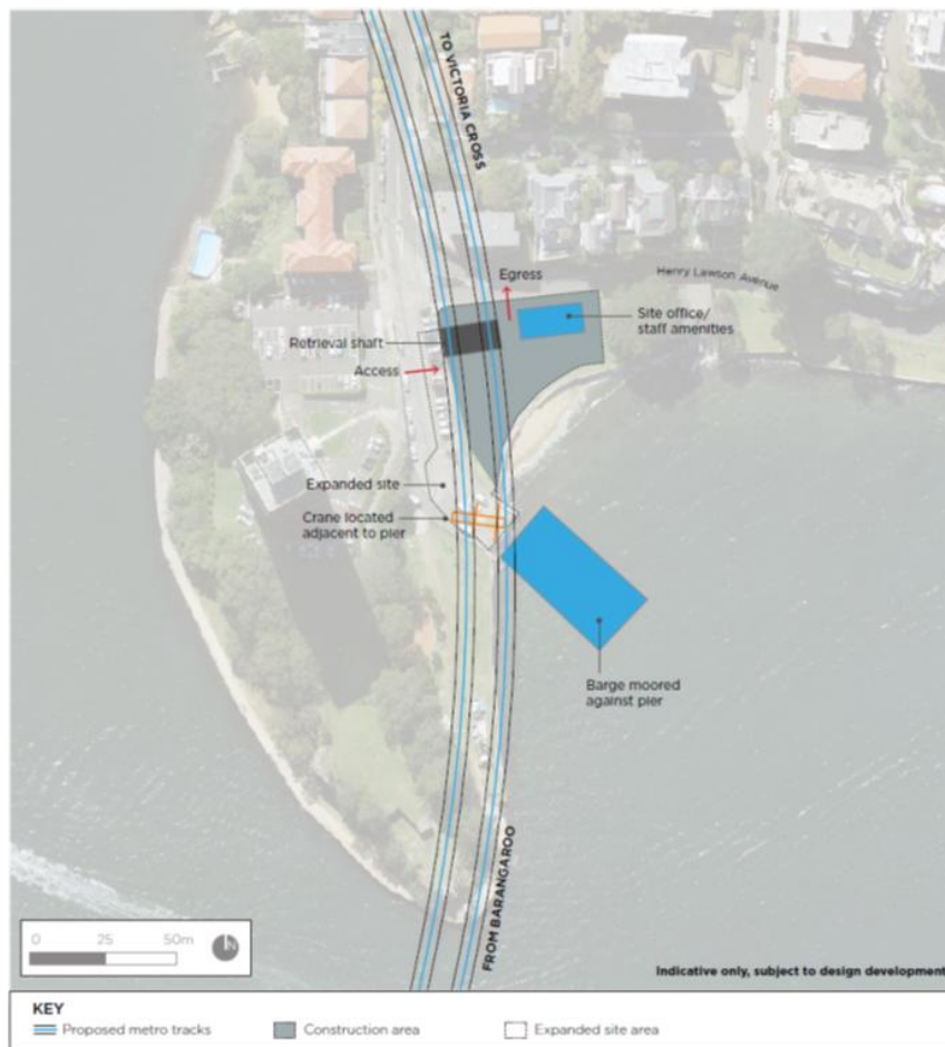
Figure 1: Potential barging arrangements at the Blues Point temporary site (extracted from the SPIR)
