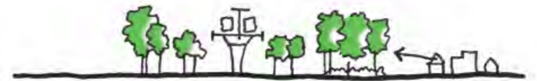
Figure 4.17_Visual Quality: Ensure screening of the viaduct from existing properties. Source: HASSELL
