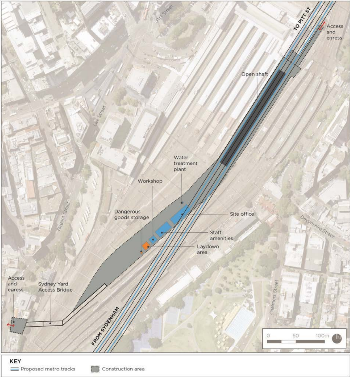
Figure 161: Central Station construction sites indicative layout.
