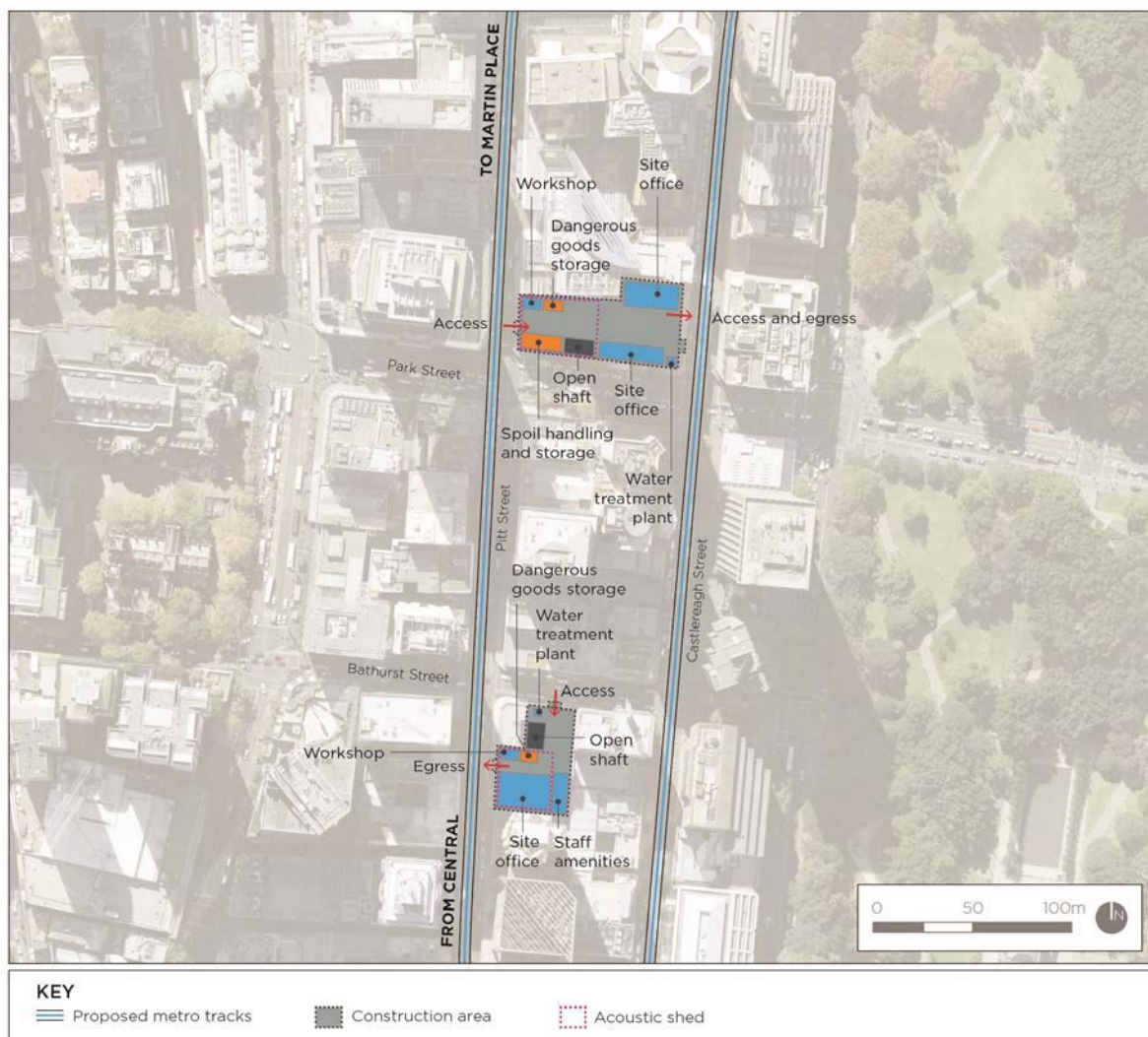
Figure 135: Pitt Street Station construction site layout.
