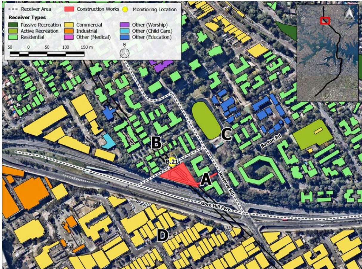
Figure 8 Artarmon Substation Construction Site and Receiver Areas
