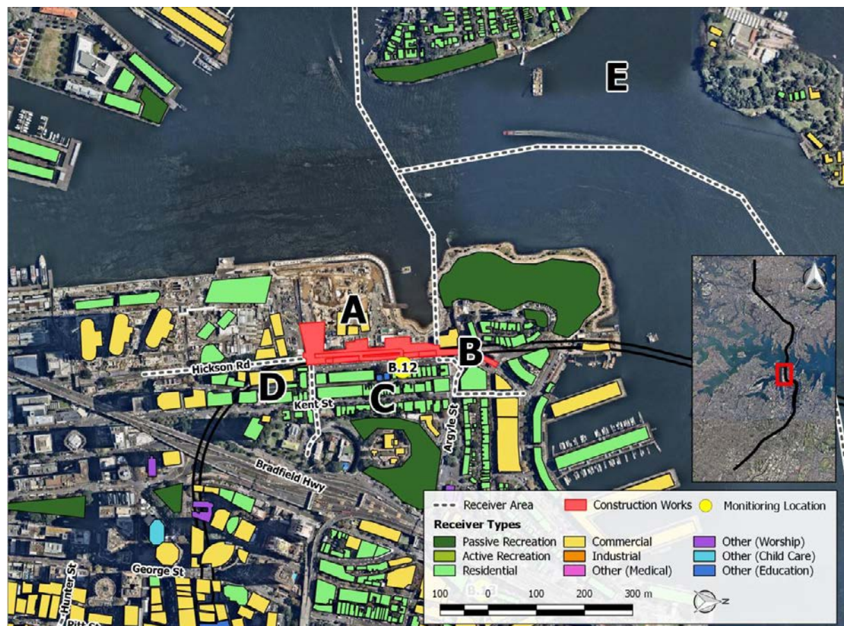
Figure 13 Barangaroo Station Construction Site and Receiver Areas
