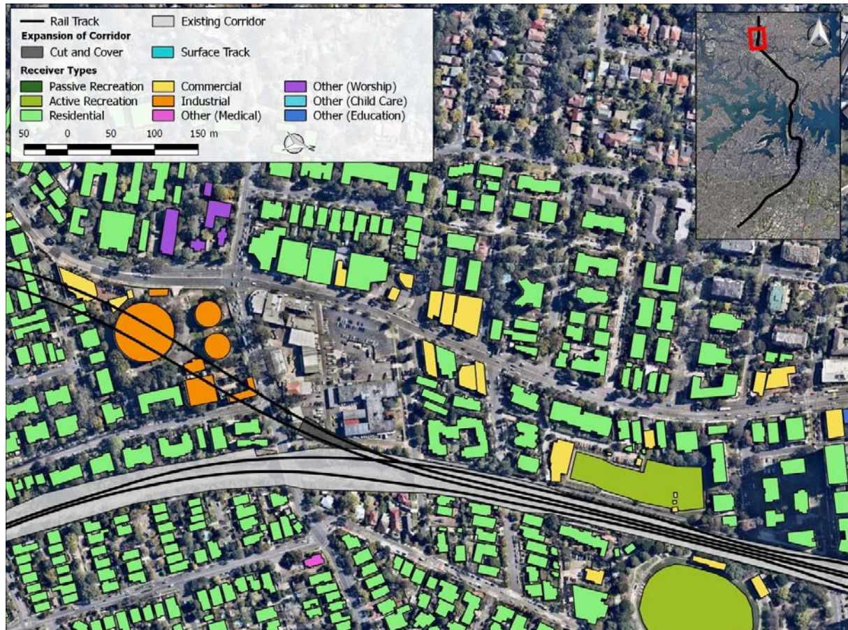
Figure 42 Corridor Widening Near Chatswood Tunnel Portal
