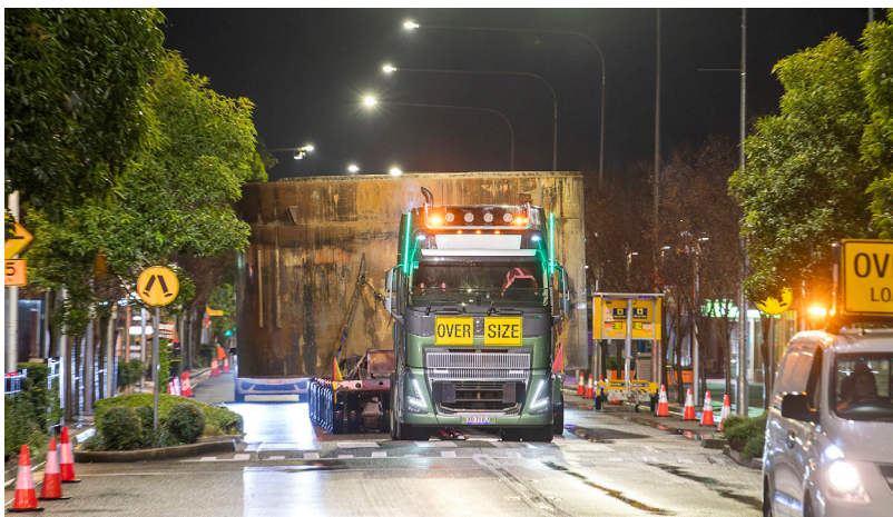
A truck transporting TBM Marlene's front shield is escorted through a narrow section of Queen Street, St Marys.
