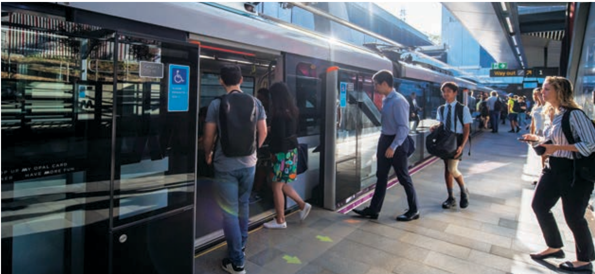
While platform screen doors are common around the world, Sydney Metro is the first Australian rail network to use them.
