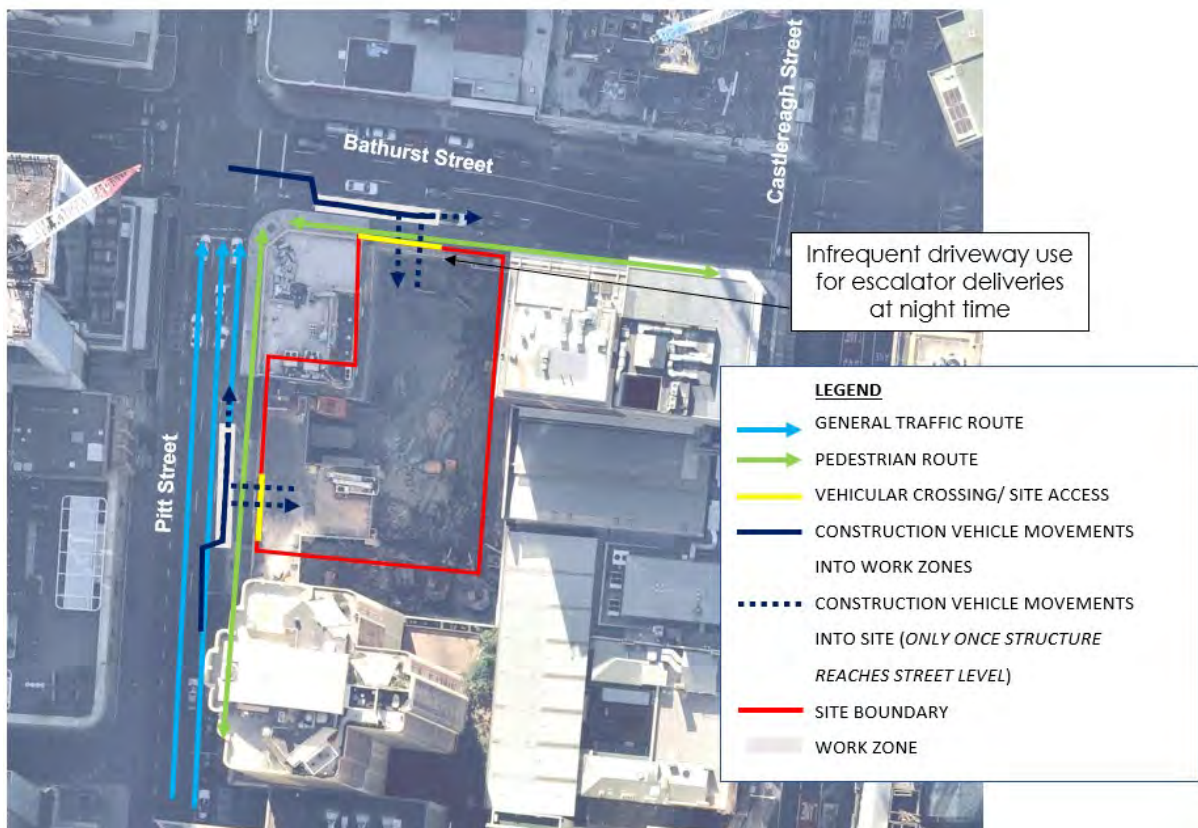
Figure 8.12: Stage 1S Indicative Traffic Staging Plan
