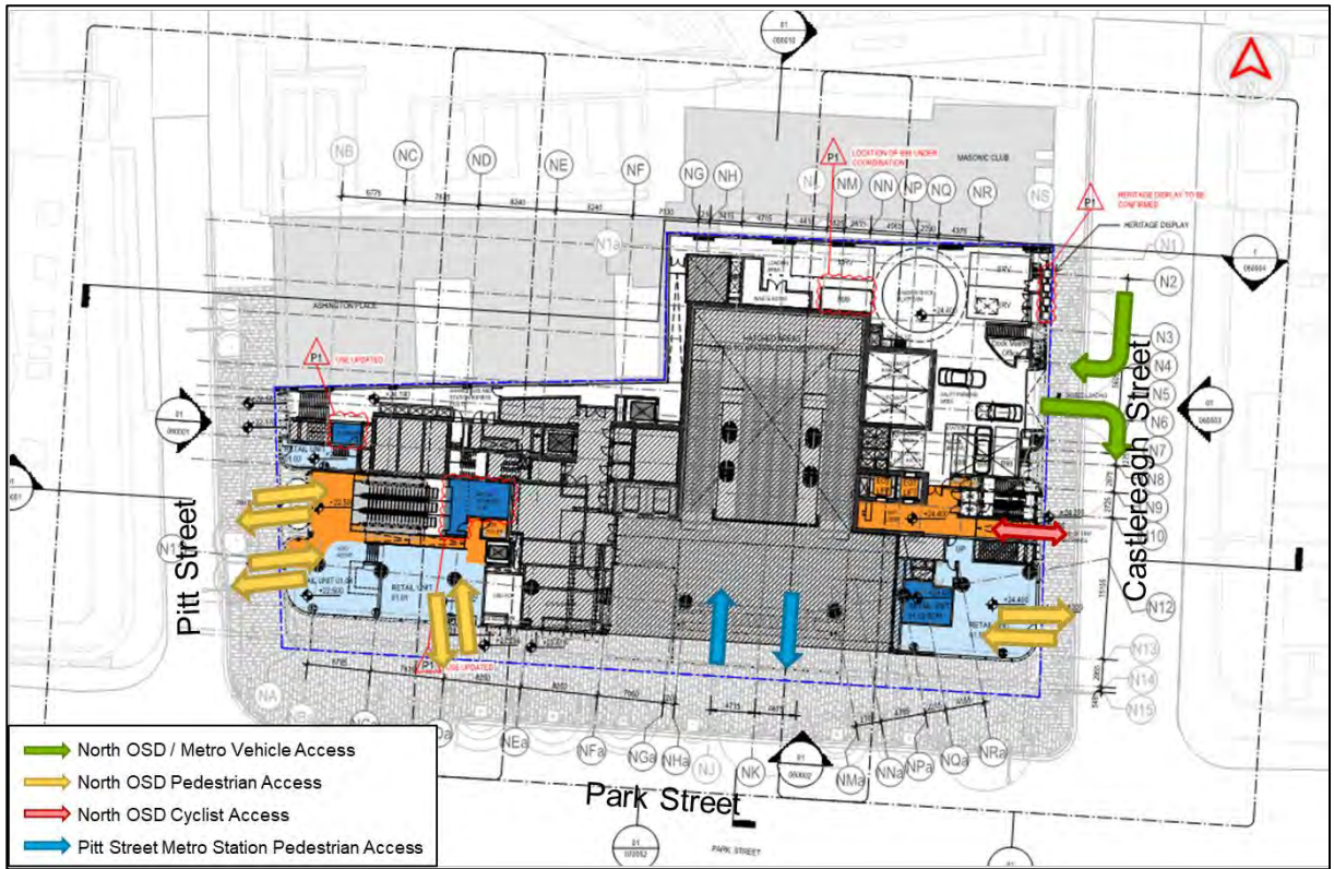
Figure 4-1: North OSD access locations on the ground floor (Reference: SMCSWSPS-FOS-OSN-AT-DWG-030013 Rev P1)
