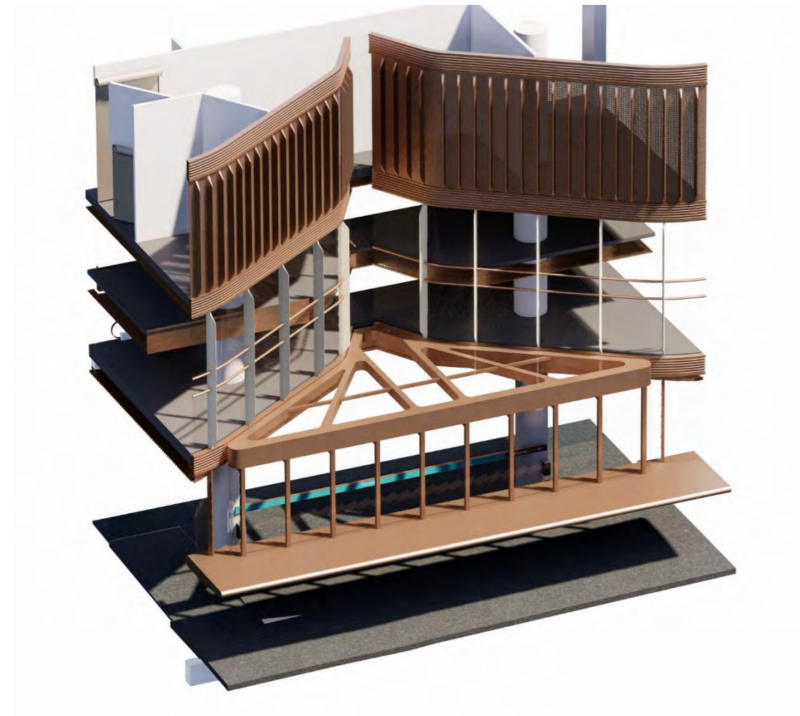
Figure 72 – North entrance external wall cladding - detail 3
