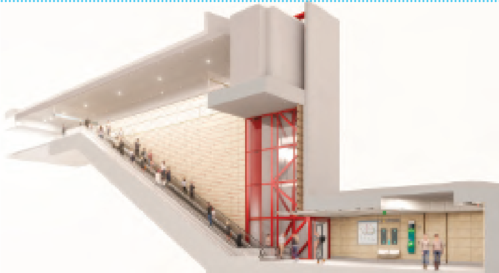
A sectional perspective illustrating the transitioning of material, colour and texture as metro customers travel from the metro station platform through the link to the existing Martin Place Station.
