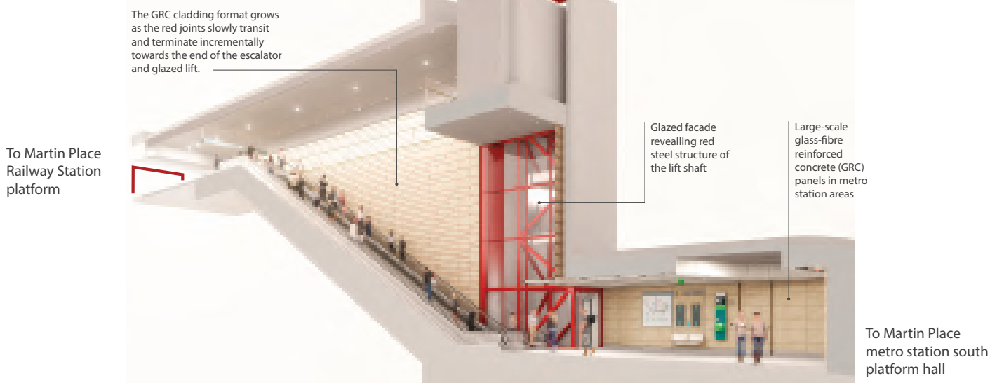
A sectional perspective illustrating the transitioning of material, colour and texture as metro customers travel from the metro station platform through the link to the existing Martin Place Station.
